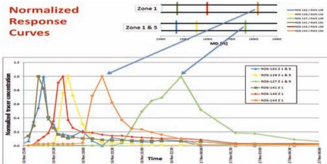
Figure 5. After a shut-in period the well was produced and tracer concentrations were measured from samples taken at the surface at five-minute intervals
