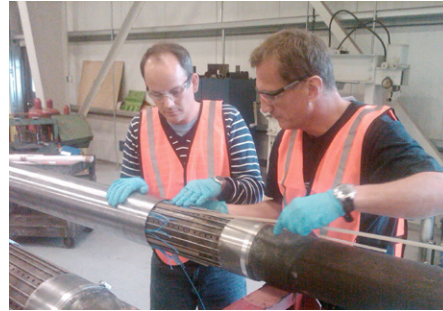
INSTALLING TRACERS IN SPECIAL DESIGNED CARRIER
