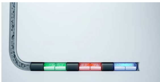
Figure 2: Well with ICD Screens Across Reservoir Interval
